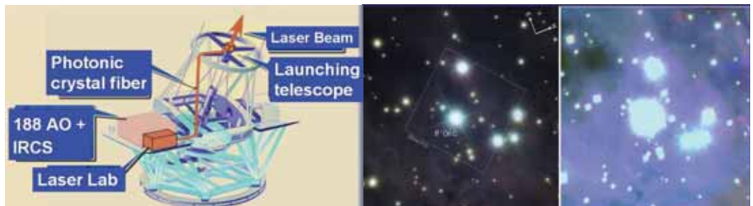
Figure 11. (a) Left: Layout of the laser, relay optical fibre, laser launching telescope, 188-element adaptive optics and instruments of LGSAO. (b).Right: Images of the Orion Trapezium, with (centre) and without (right) AO.
