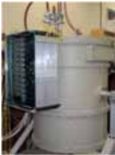
Figure 9. AzTEC cryostat and readout electronics.
