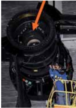
Fig. 13. Prime focus corrector for FMOS
