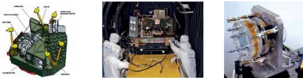
Figure 12. The FGS-TF instrument layout (left), test unit in space simulation chamber (center), and prototype Fabry-Perot etalon (right).
