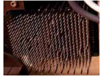
Fig.14 Fibre spine heads of Echidna. Fibre positioner.
