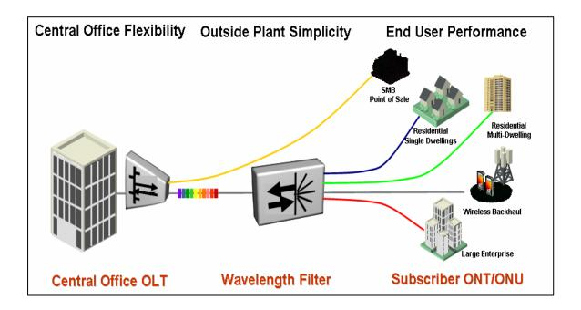
In WDM PON, a single wavelength is re-directed to an end user from the central office via a passive wavelength router located in the outside plant (OSP). Unlike
