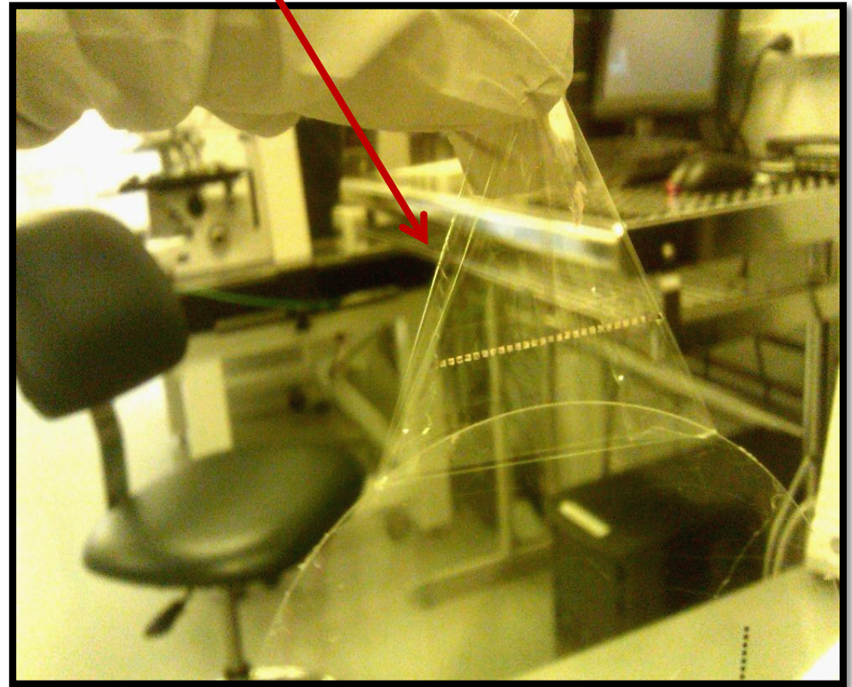
Parylene C – 4 \mu\text{m} thick
